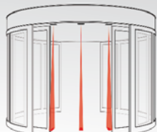
Curved sliding doors Safety during the closing cycle
