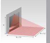
Example of detection zone: H = 5 m W = 6 m D = 7.5 m(calculation matrix  $64 \times 64$ )
