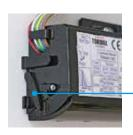
Depth adjustment for motion detection
